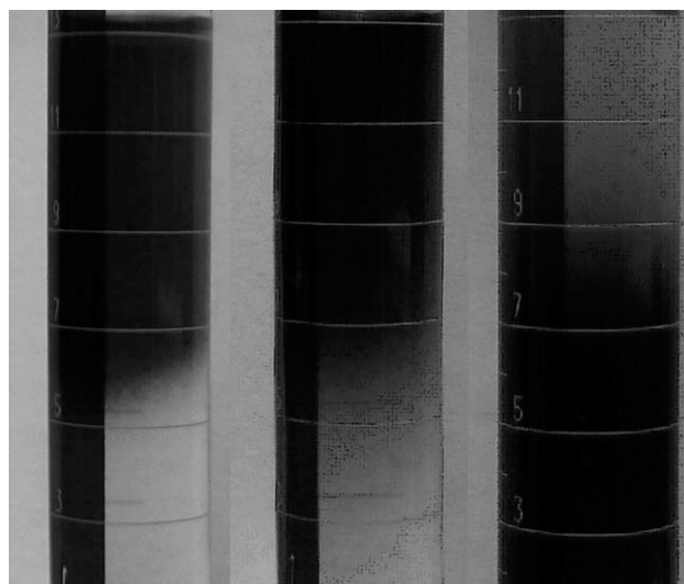
Figure 1 Visual determination of diffusion in the 0.3% saponified starch–polyacrylonitrile gel. The photographs were taken at 1 day (left) and 9 days (middle). An analogous experiment with the die layer on the bottom is also shown after 9 days (right).
